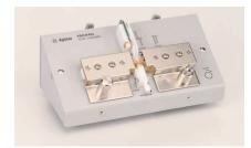
A chip component test fixture with 4-terminal configuration suited for measurement of low impedance devices such as high-value capacitors. Built-in arm-type terminators make it possible to configure appropriate terminal connections easily and quickly for Open/Short compensations by simply turning the arms.
